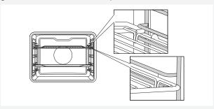
With telescopic extendible guides, first pull out the guides of one level and place the grid or the baking tray onto them. Then, push them in with your hand as far as they will go.
