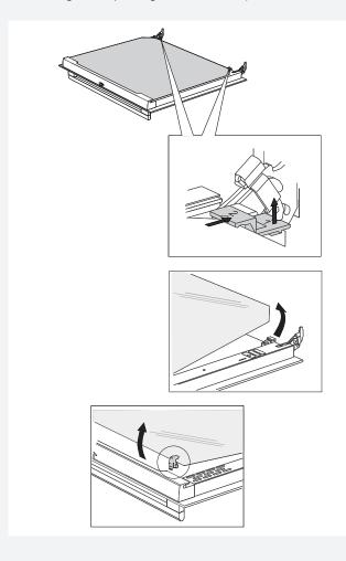
Slightly lift the supports on the left and right side of the door (marking 1 on the support) and pull them away from the glass pane (marking 2 on the support).
