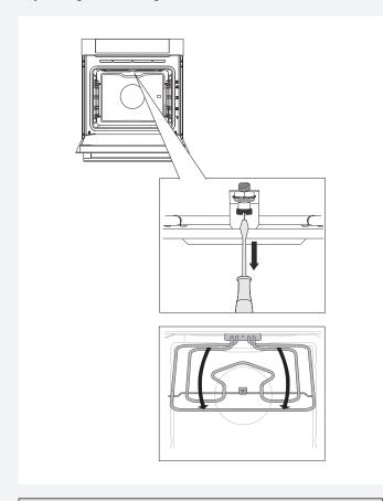
To remove the heater, undo the screw located at the front of the oven cavity ceiling.
