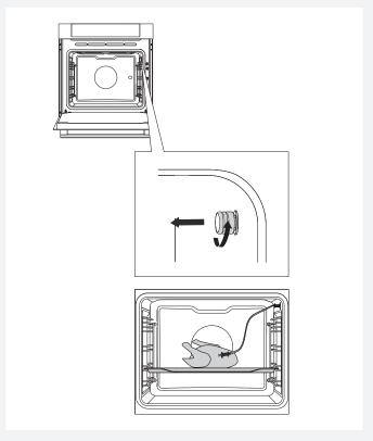
Remove the metal cap (the socket is in the front upper corner of the oven right wall).
