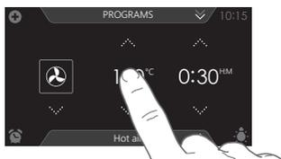
1. Tap in the centre of the function symbol, temperature, power or cooking time (activated). The keyboard appears.
