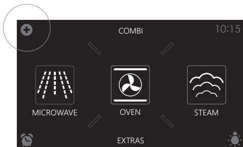
The 'Plus' menu comprises a number of functions or settings. The offered plus functions depend on the display that is active.
