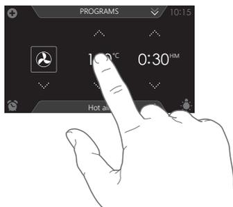
1. Tap in the centre of the function symbol, temperature or cooking time (activated). The keyboard appears.
