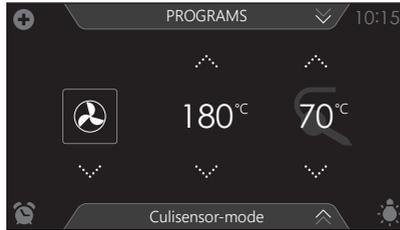
4. Select an oven function, temperature and core temperature (see 'Function-setting display' chapter).
