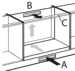
Ventilation occurs through the plinth (A) and the back of the cupboard (B). Saw out the ventilation openings (min. 100 cm<sup>2</sup>). Air supply A is superfluous when, together with opening B, there's an opening somewhere else where air can be drawn in.
