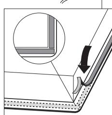
Remove the protective layer from the sealing tape and apply the tape in the groove of the aluminium profile or on the edge of the glass plate. Do not stick tape round the corners, but cut 4 separate pieces to seal the corners well.
